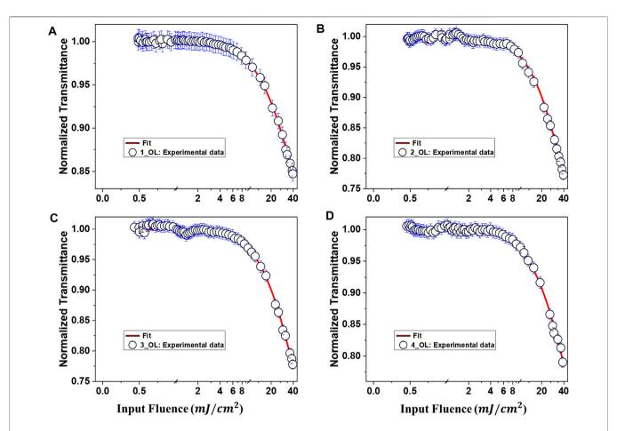
FIGURE 5 | Optical-limiting behavior of uGFPc (A) 1, (B) 2, (C) 3, and (D) 4 and in DMF solution as a function of input laser fluence with fs pulse excitation. Theoretical fits to the experimental data (open symbols) are indicated by solid lines.
