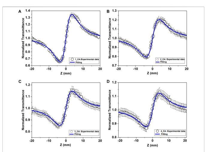
FIGURE 4 | Closed-aperture (CA) Z-scan curves for the samples (A) 1, (B) 2, (C) 3, and (D) 4 obtained with 800 nm, 70 fs pulses. Open symbols are the experimental data points, while solid lines are theoretical fits.
