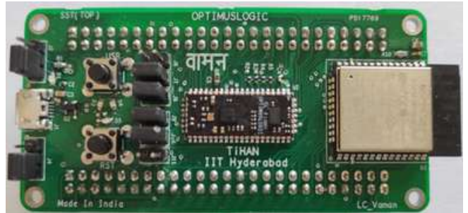
Figure 16: TiHAN-IIT Hyderabad OptimusLogic "Vaman" Board
