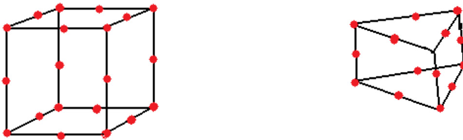
Fig 2.3 Twenty noded solid element in brick and prism type with red dots indicating the nodes
