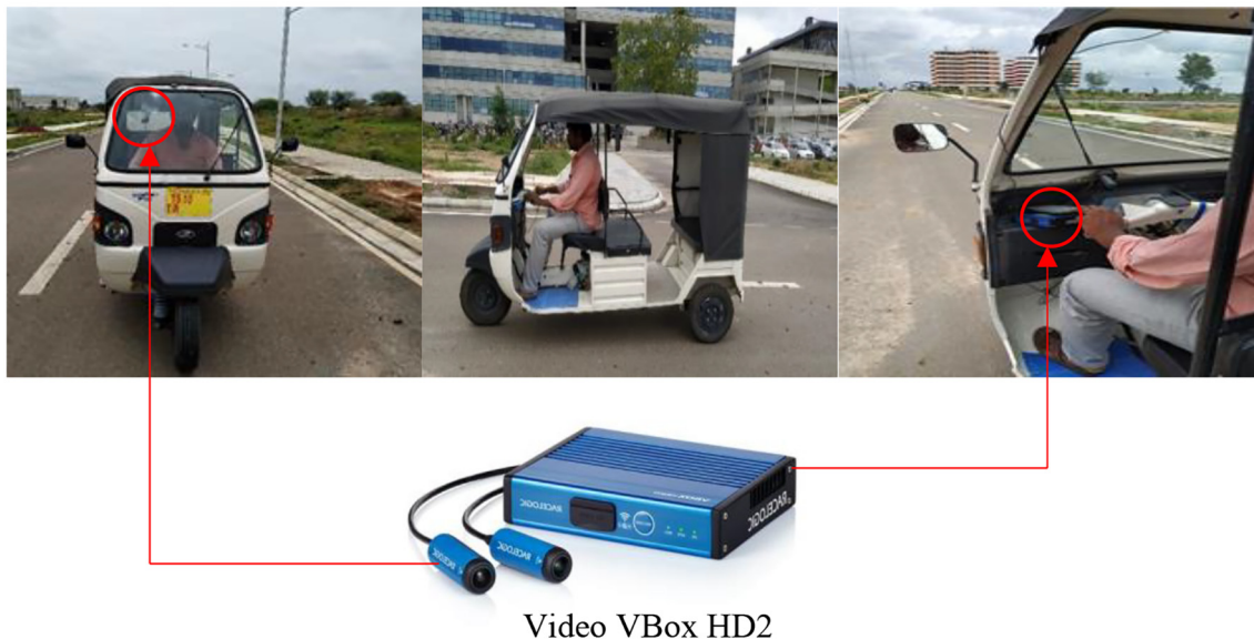
Fig. 2. Instrumented test vehicle used for the study.
