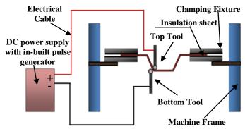
Fig 1: Schematic of experimental set-up used for Incemental Electro-plastic deformation
