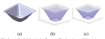
Fig 5: (a) CAD Model (b) Contour Tool path (c) Helical Tool path
