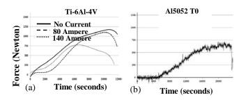
Fig 8: (a) Load measurement for 30 degree truncated pyramid of Titanium alloy (frequency: 55 Hz, On-time: 3ms, Max. temp: around 47° C with 140amps current) (b) Load curve for 30 degree truncated pyramid of Al5052T0 without electro-pulsing
