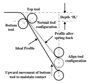
Fig 13: Mixed tool configuration
