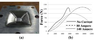
Fig 14: (a) Actual picture of 45° pyramidal component formed at 140 ampere current (b) Force data for 45° pyramidal component at 0, 80 and 140 ampere current
