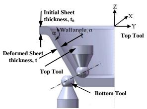
Fig 4: Normal tool configuration
