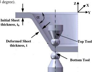
Fig 12: Align Tool Configuration
