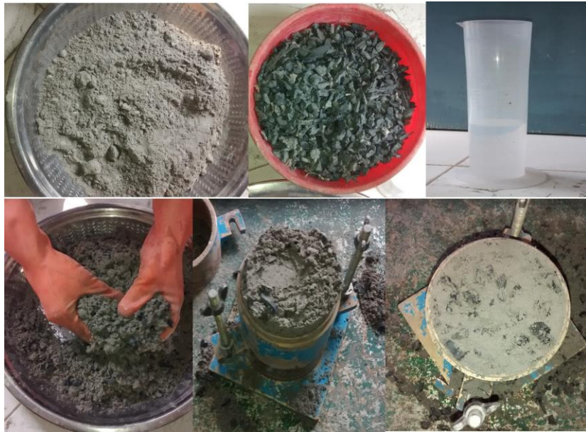
Fig 3.14 Preparation of fly ash and tire chip mixtures during standard Proctor compaction test
