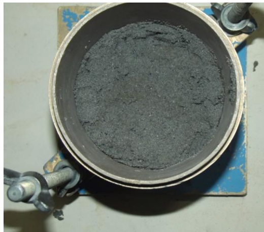
Fig 3.9 Photograph of compacted first layer of sample in 100mm-diameter mould
