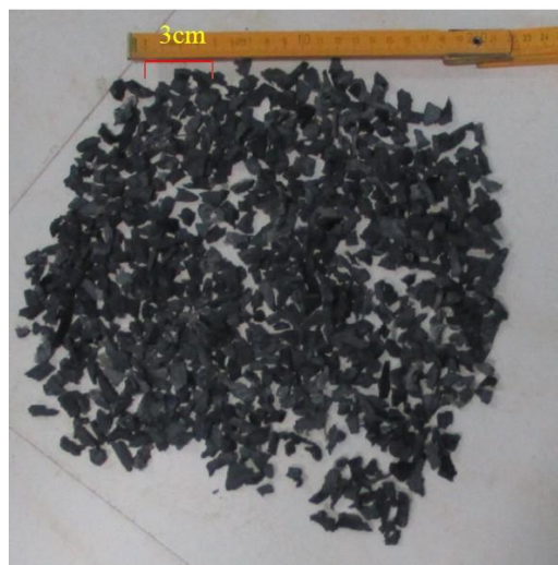
Fig 3.5 Photograph of tire chips used in the study
