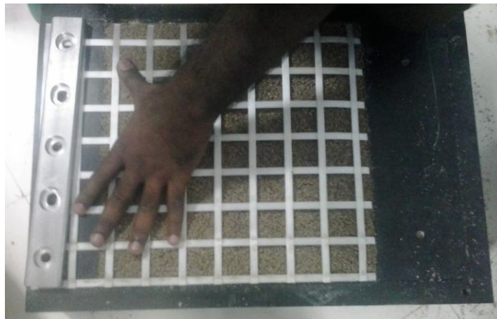
Fig 3.12 Placing of geogrid on top of compacted sample in the lower shear box
