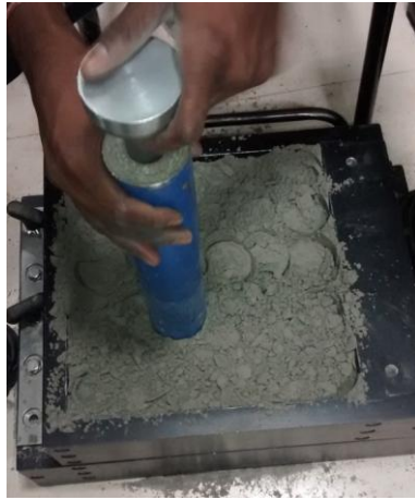
Fig 3.10 Sample preparation in the direct shear box
