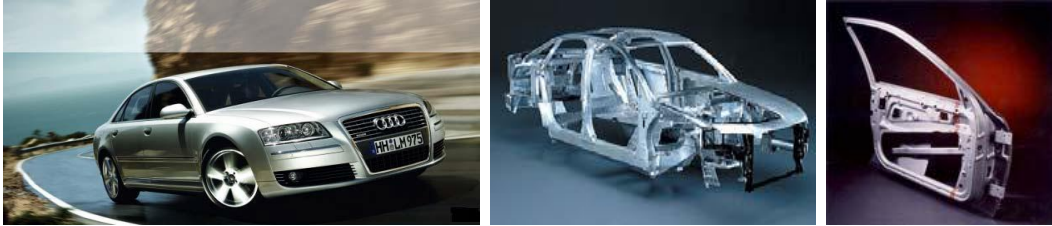
Figure-12: Audi A8 with an aluminium space frame and tailored blank door structure for weight reduction [48].
