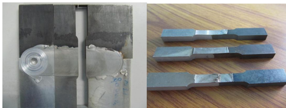
Figure. 7. Tensile specimens cut from EDM
