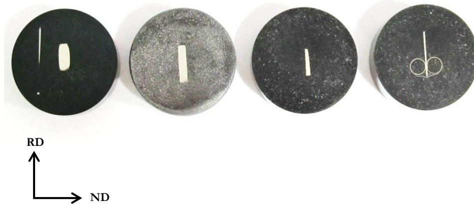
Figure 3.3.1: The mounted specimen with RD-ND plane at top for hardness test, Mounted specimens: SCR 20%, SCR 40%, SCR 65%, and SCR 90% (from left to right).
