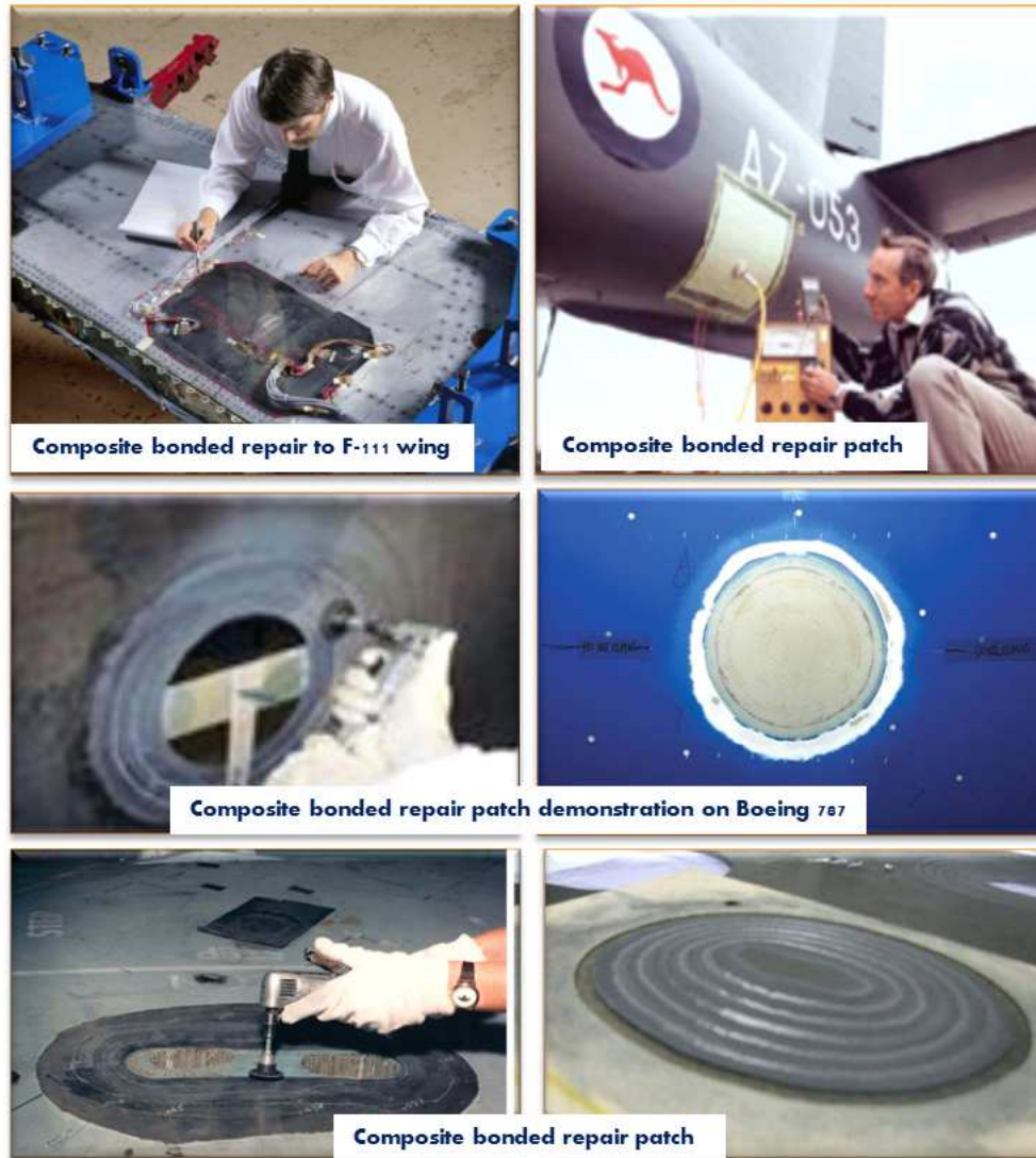
Figure 1.10: Application of bonded patch repair on an aircraft [8]
