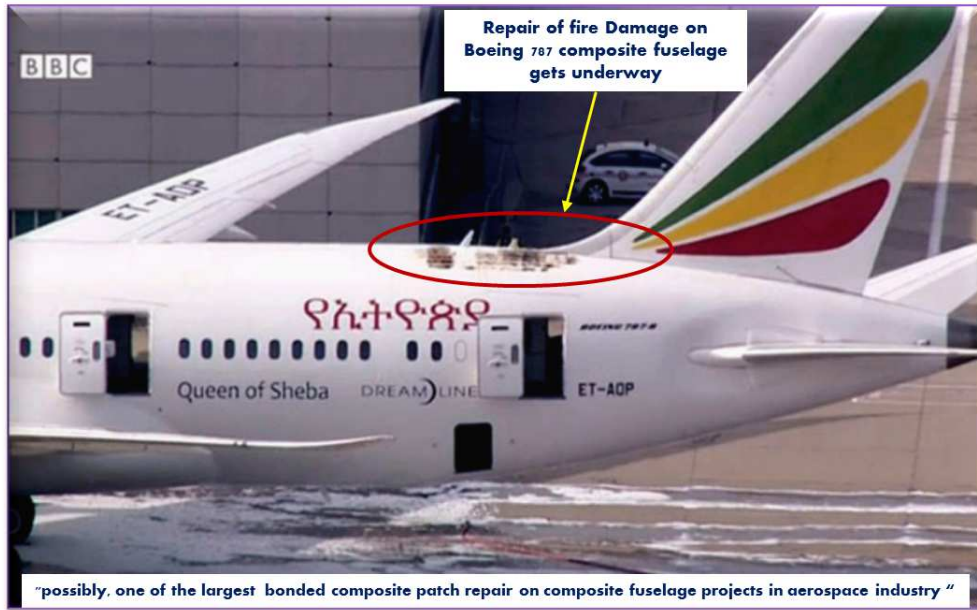
Figure 1.9: Damage on composite fuselage of Boeing 787 Dreamliner aircraft whose repair process utilizing adhesively bonded patch is underway [7]
