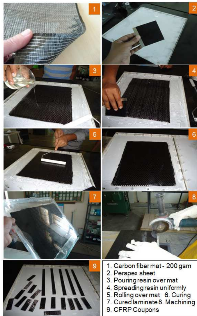
Figure 2.1: Different steps involved in CFRP specimen preparation
