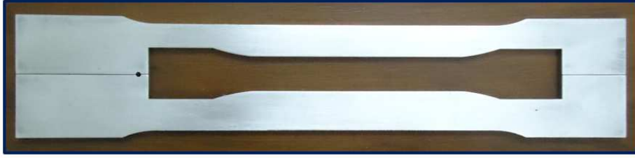
Figure 5.1: Split aluminium mold used for casting of adhesive specimens
