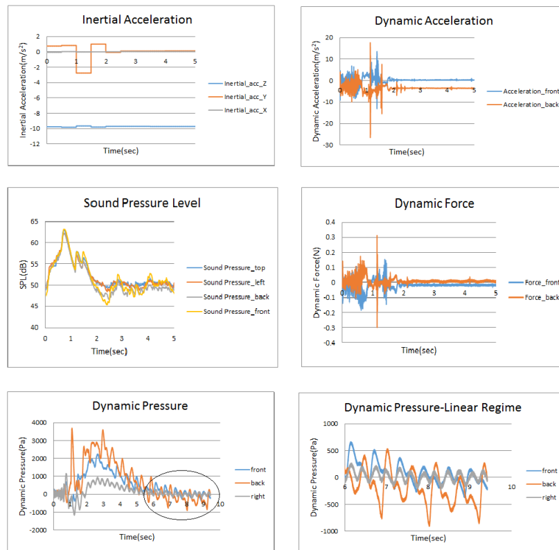
Figure 5.22: Experimental results for 60 % fill and 0.25 g deceleration and sensor height 50 % case (a) Inertial acceleration (b) Dynamic acceleration (c) SPL (d) Dynamic Force (e) Dynamic pressure (f) Linear regime in sloshing
