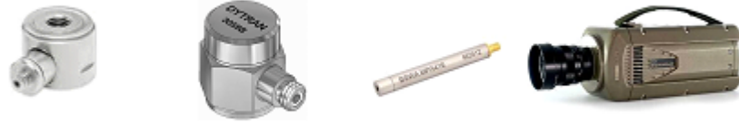
Figure 3.11: Sensors used for data acquisition (a) Dynamic force (b) Dynamic acceleration (c) Microphones (d) High speed camera
