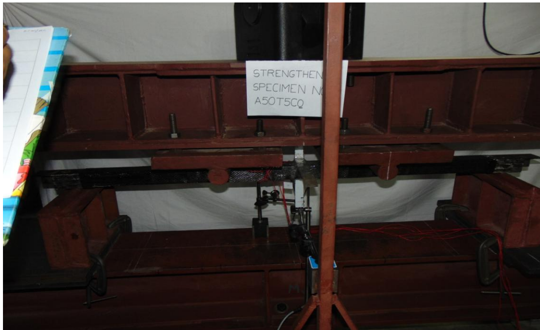
Figure 4.20: Specimen no. 30 under four point bending test setup
