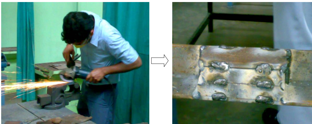
Figure 3.5 : Grinding of plates and intermittent welding
