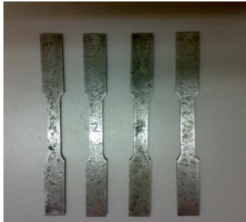
Figure 3.3: Finished tensile test coupons
