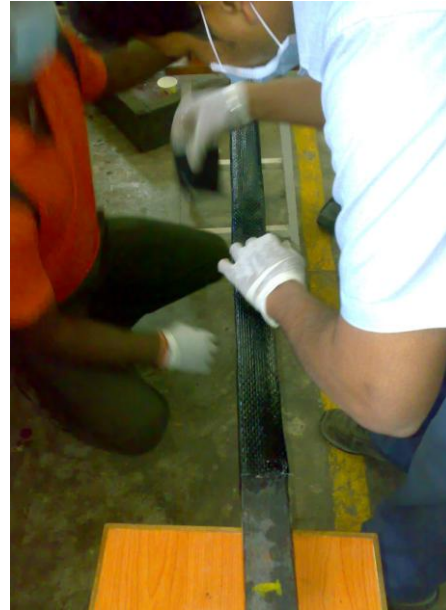
Figure 3.16 : CFRP wrapping (Second layer unidirectional)
