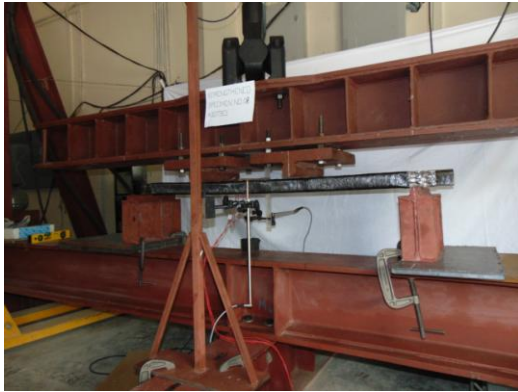
Figure 4.6 : Specimen No.4 under four point bending with LVDT's at marked location
