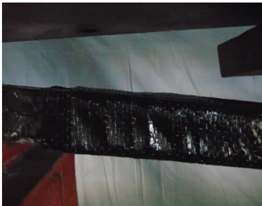
Figure 4.8 : Specimen No.4, debonding and delamination in shear zone (enlarged view)
