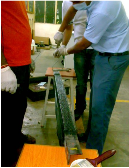
Figure 3.15 : CFRP wrapping (single layer unidirectional)
