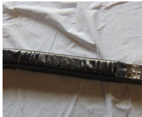
Figure 4.8 : Specimen No.4, debonding and delamination in shear zone (enlarged view)
