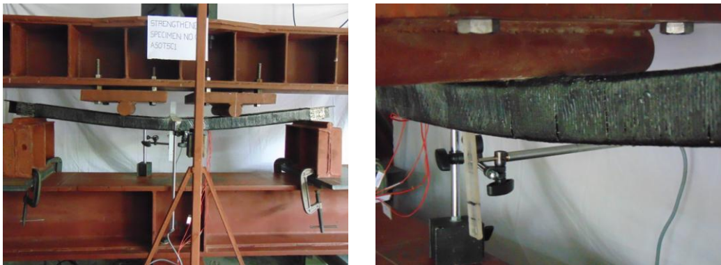
Figure : Delamination and debonding in flexure-shear zone
