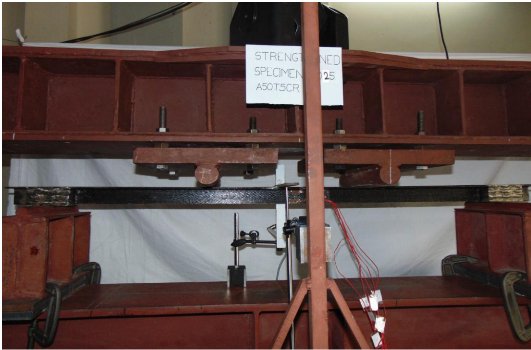
Figure 4.17: Specimen No. 25 under four point bending test setup
