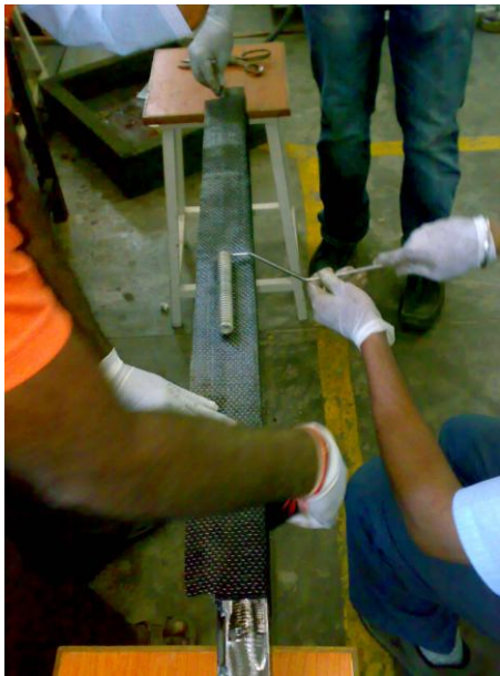
Figure 3.16 : CFRP wrapping (Second layer unidirectional)
