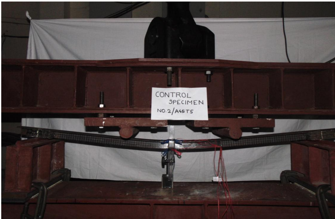
Figure 4.3 : View of Flexural Yielding (FY)
