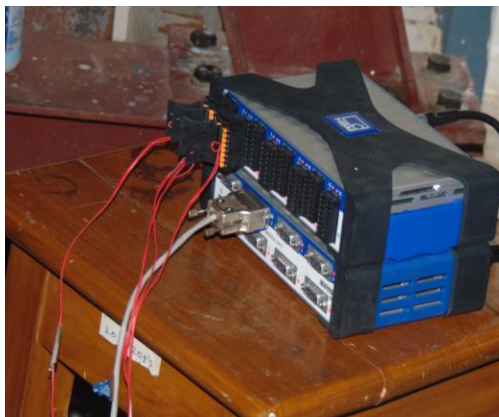
Figure 3.23 : HBM DAQ and HBM Controller Computer
