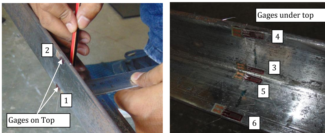
Figure 3.24 : Strain gauge location Type-1
