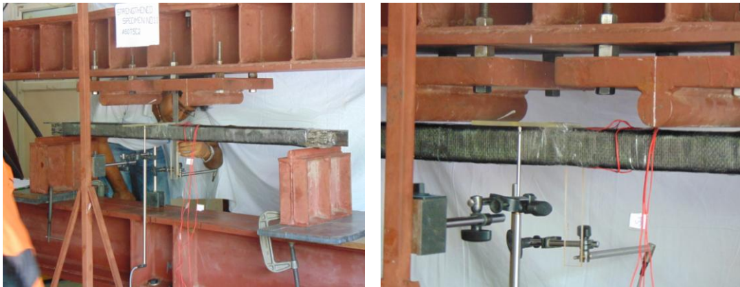
Figure 4.11: Intact CFRP wrapped specimen no. 7 before loading
