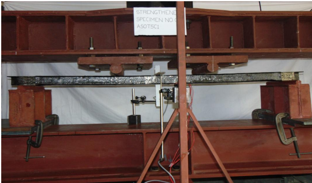
Figure 4.9 : Specimen No.19 under four point bending
