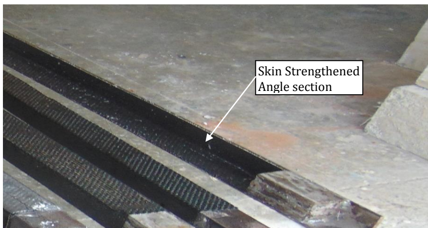
Figure 4.16: Skin Strengthened Angle section [0]
