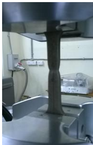
Figure 4.52: Tensile coupon test onset of fracture
