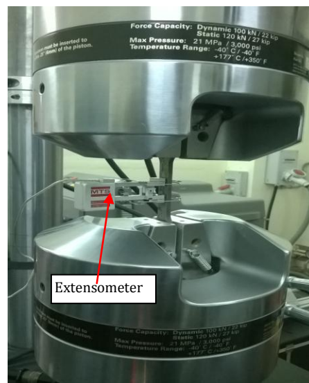
Figure 3.27 : Tensile specimen with extensometer attached
