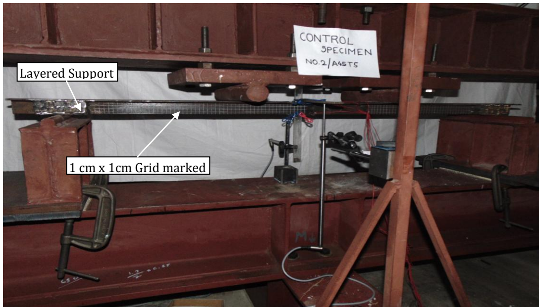
Figure 4.1 : Control specimen under four point bending
