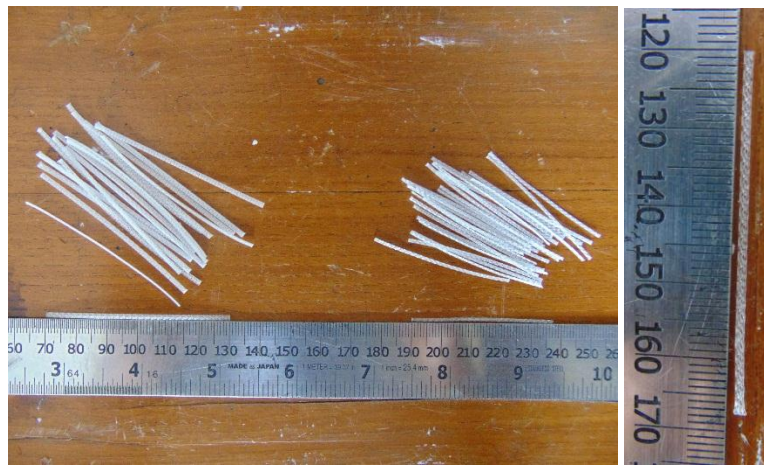
Figure 3.1: FibreTuff™ Monofilament structural polypropylene fiber
