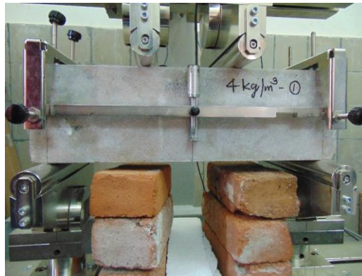
Figure 3.2: Test setup as per ASTM C 1609
