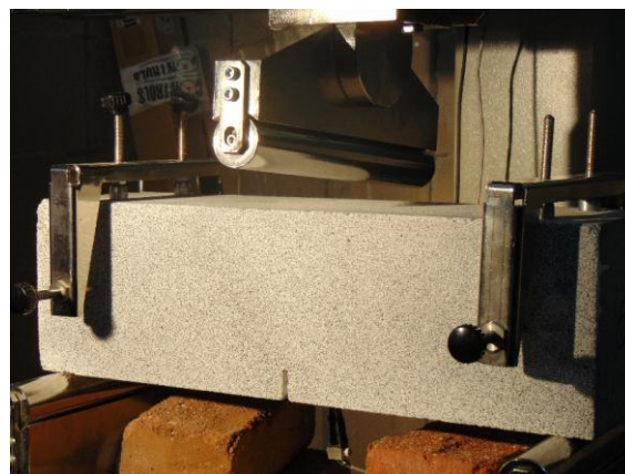
Figure 3.3: Test setup as per EN 14651-2005
