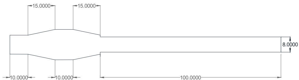
Figure 43 : Tapered tool used for conventional cold expansion
