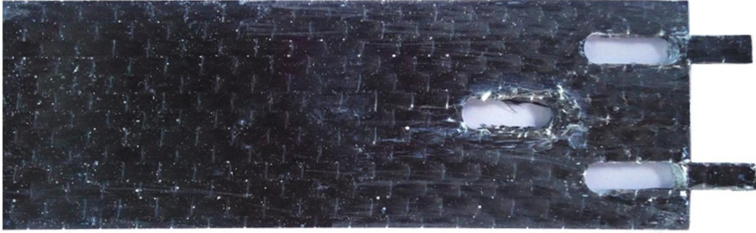
Figure 3.8: Image showing final failure of the middle panel
