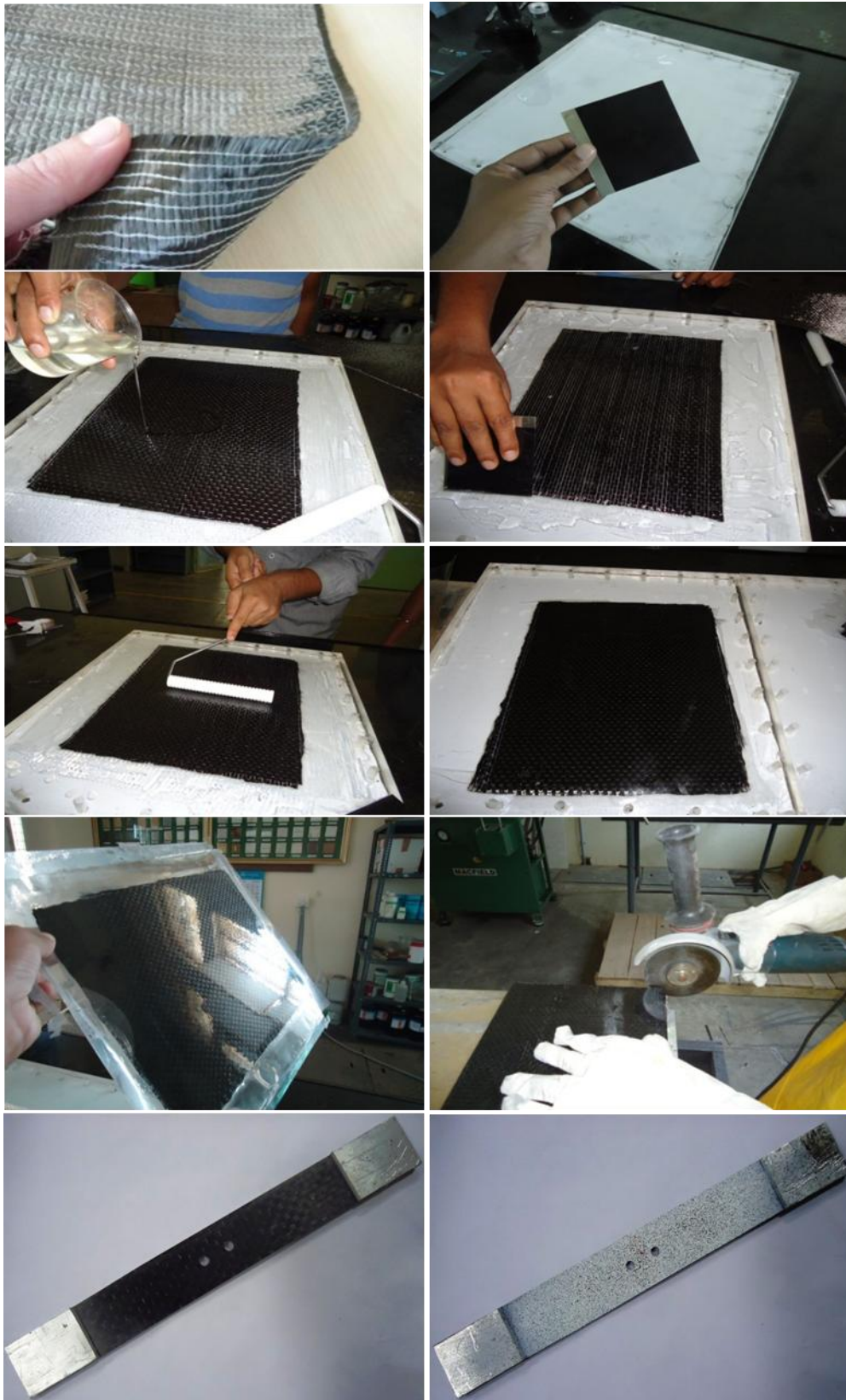
Figure 2.2: Different steps in CFRP specimen preparation
