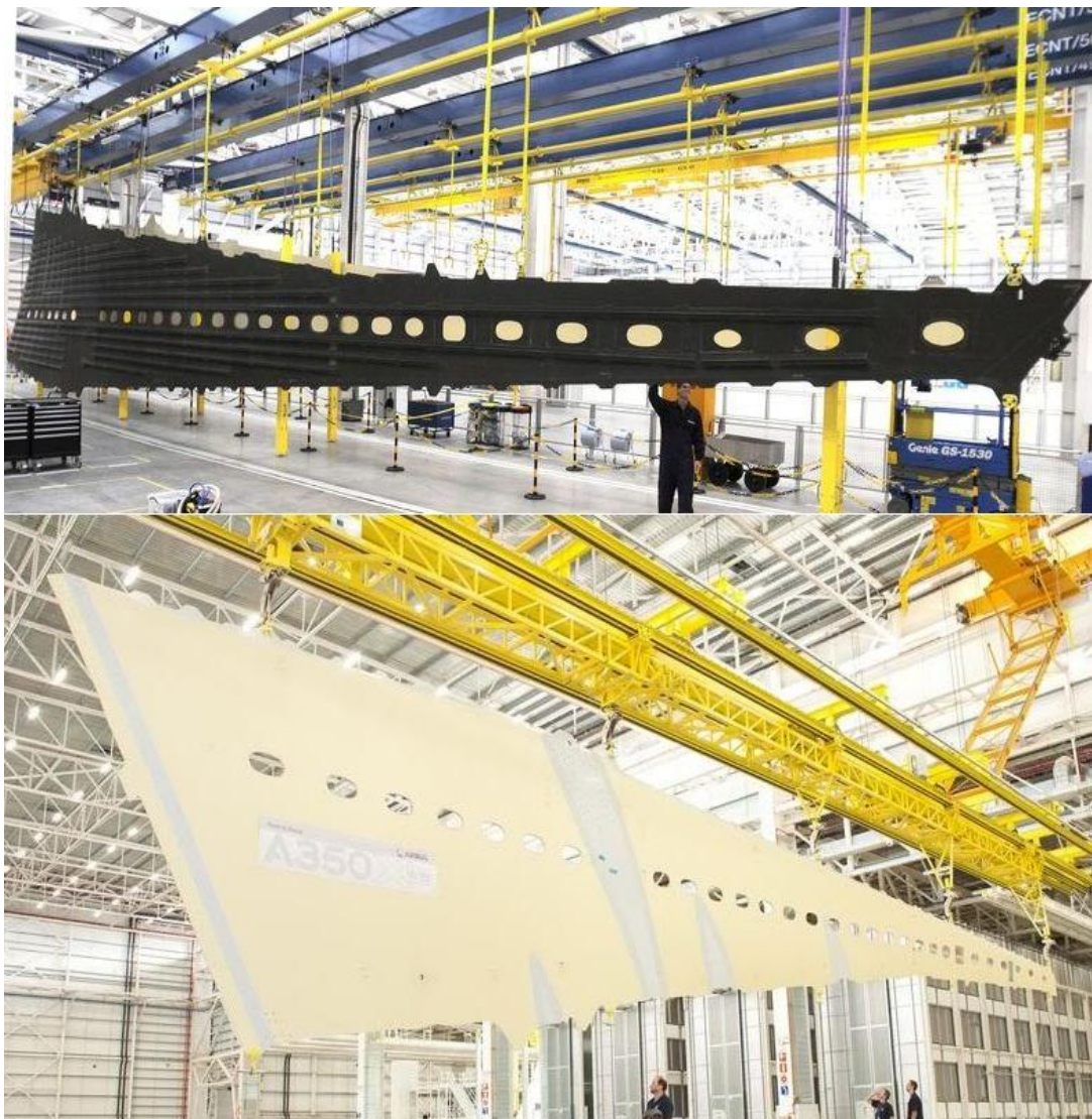
Figure 1.3: Wing covers of Airbus A350 XWB made of CFRP [2]
