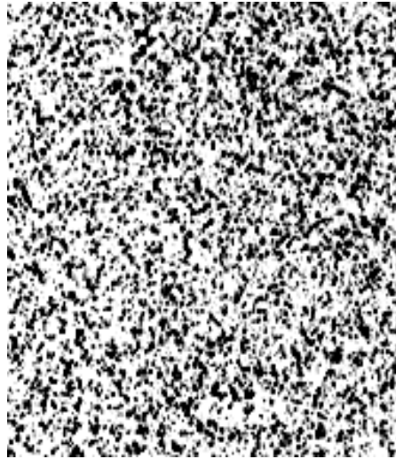
Figure 1.8: A typical random speckle pattern applied over the specimen.
