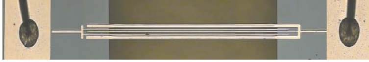
Figure 3.2: A picture of 3-beams array with two side electrodes and a bottom electrode.
