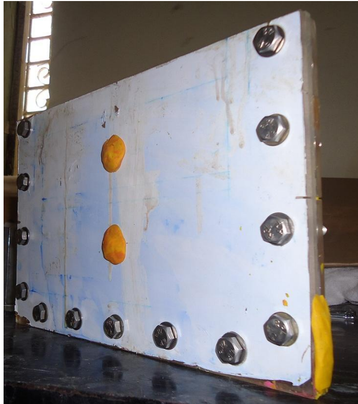
Fig. 3.3 Mould used for preparing crack inclusion specimens
