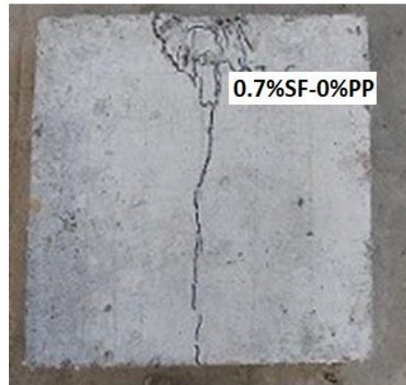
Figure 9. Failure of the panel with 0.7% macro steel fibres only
