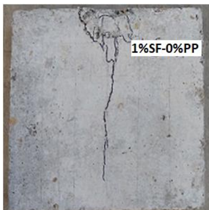
Figure 12. Failure of the panel with 1% macro steel fibres only
