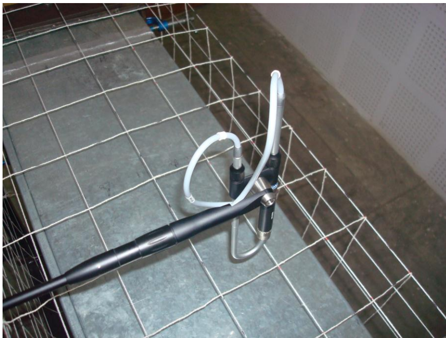
Figure 3.20: Sound intensity probe orientation over the scanning the virtual surface.
