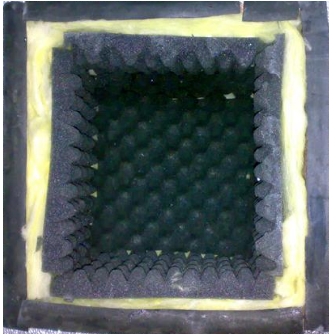
Figure 3.7: Enclosure with absorptive material on the inner walls and isolator on enclosure edges.
