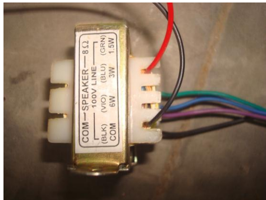
Figure 3.8b: Speaker transformer with power tapping
