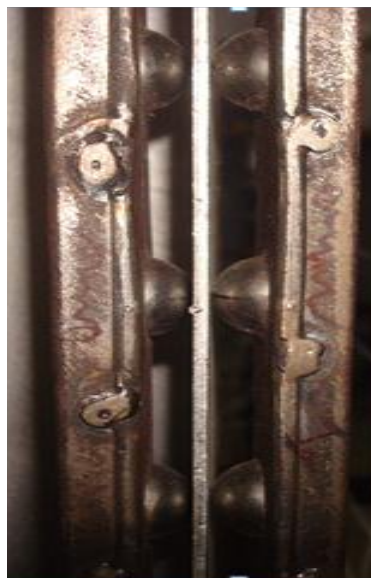
Figure 3.4c: Simply-Supported frame with steel balls in point contact
