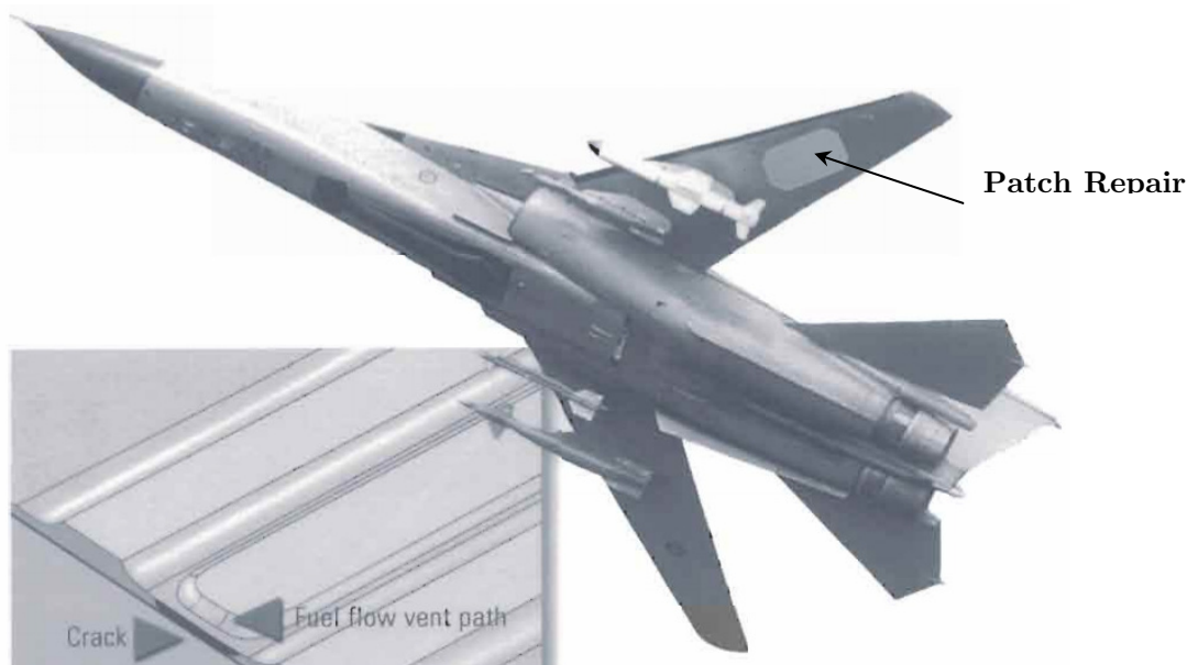
Figure 1.2: Application of patch repair to the wing of F-111 military aircraft [1]
