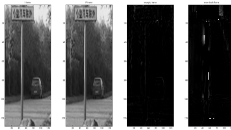
Figure 7.7: Image frames, error frames of image and depth map using motion vectors of image. Corresponding autocorrelation values are R_{image}(0) = 54.56 R_{depth}(0) = 1892.85
