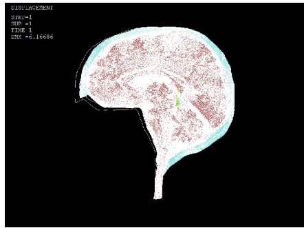
Figure 2-8: Displacement with No. of elements 205411
