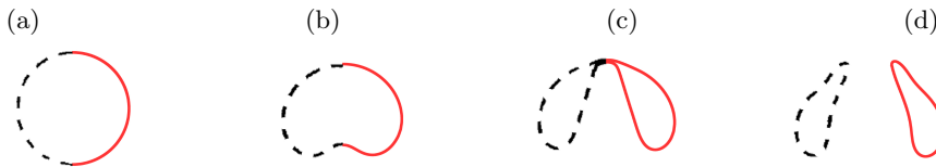
Figure 3: Comparison of the evolution of the shape of the bubble obtained from our simulation (shown by red line) with Sussman & Smereka (1997) (dashed line) at various times in an isothermal system: (a) t = 0 , (b) t = 0.8 , (c) t = 1.6 and (d) t = 2.4 . The parameter values are Ga = 100 , Bo = 200 , \rho_r = 10^{-3} and \mu_r = 10^{-2} .
