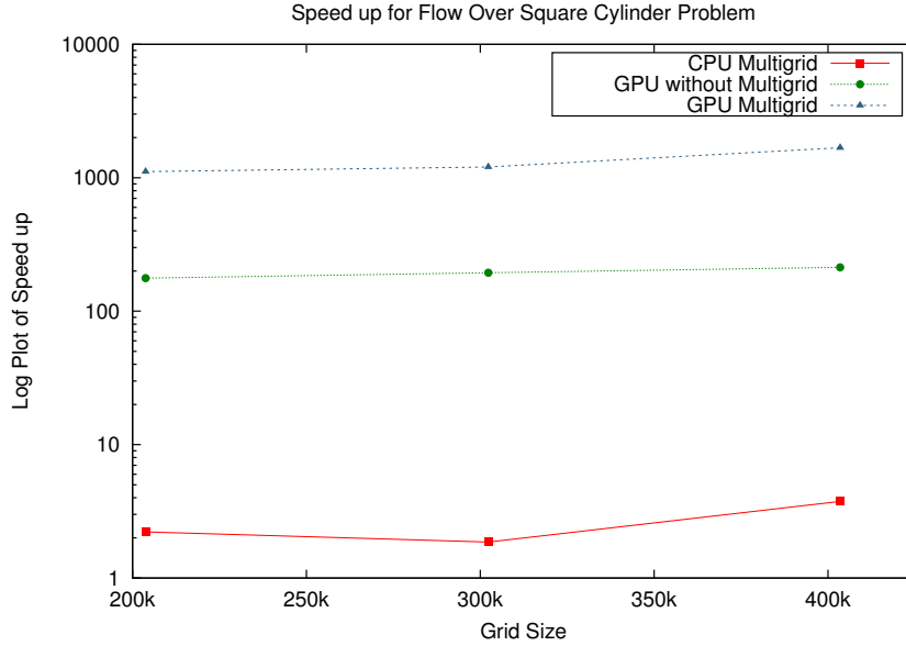
Figure 6.13: Pressure Poisson solve time speed up comparison for laminar flow past square cylinder problem
