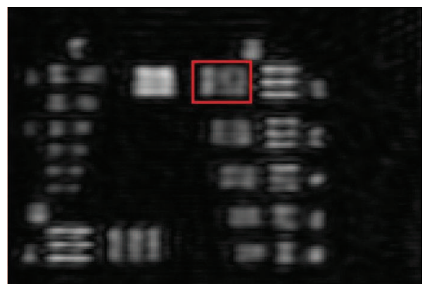
Figure 4-20 Zoomed version of amplitude reconstruction single hologram of USAF resolution chart
