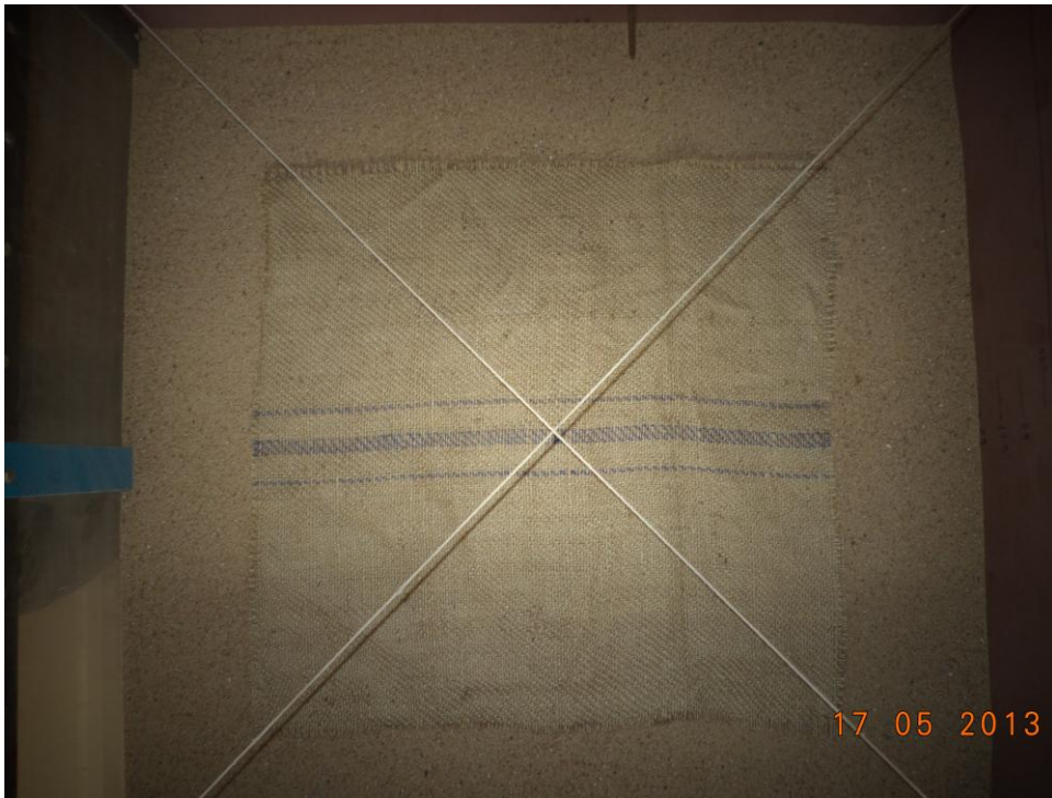
Figure 4.6 Typical placement of geojute layer in the test tank
