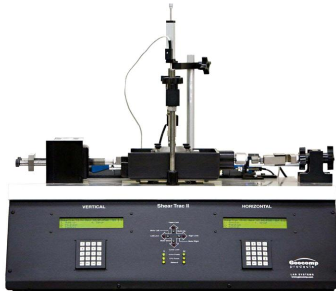
Figure 3.2 Direct shear test apparatus
