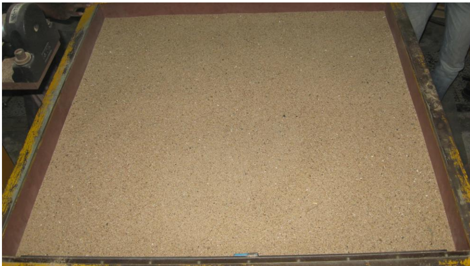
Figure 4.7 Typical leveled sand bed before the test
