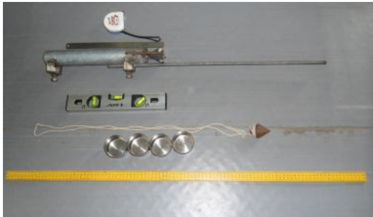
Figure 3.12 Devices used in the preparation of bed
