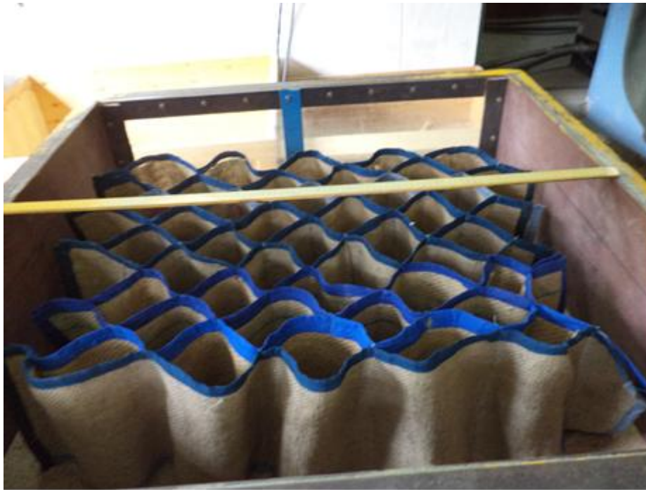
Figure 5.2 Hand-made jute-geocell used in the study
