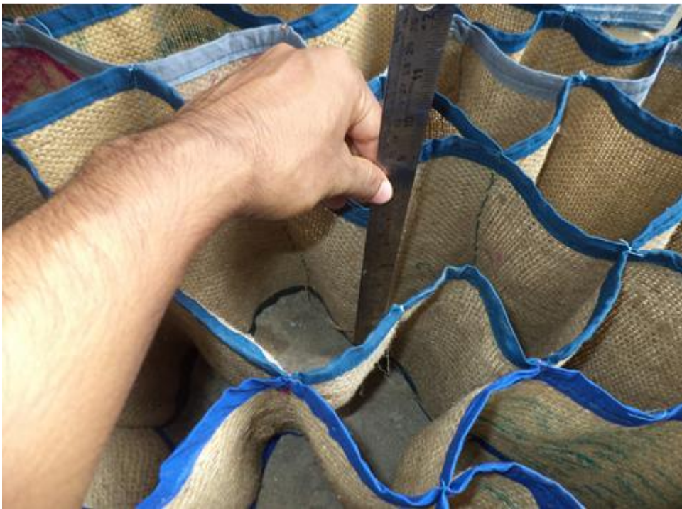
Figure 5.10 Weld Failure in Jutegeocell (Series-G 3 )
