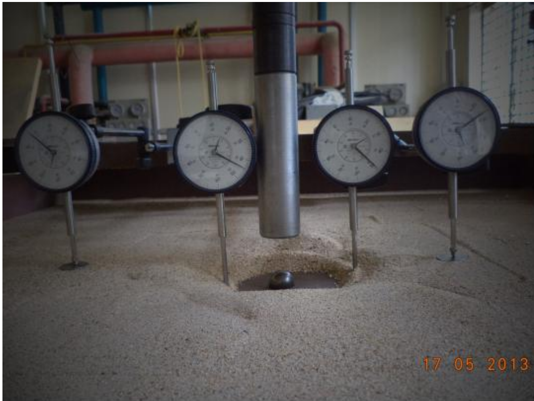
Figure 5.6 Plate and Surface deformations after the test
