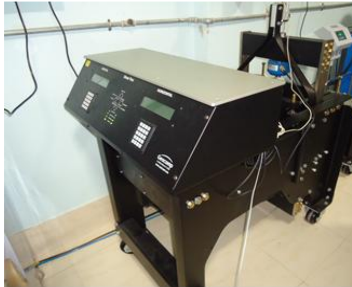
Figure 3.5 Large-scale direct shear apparatus
