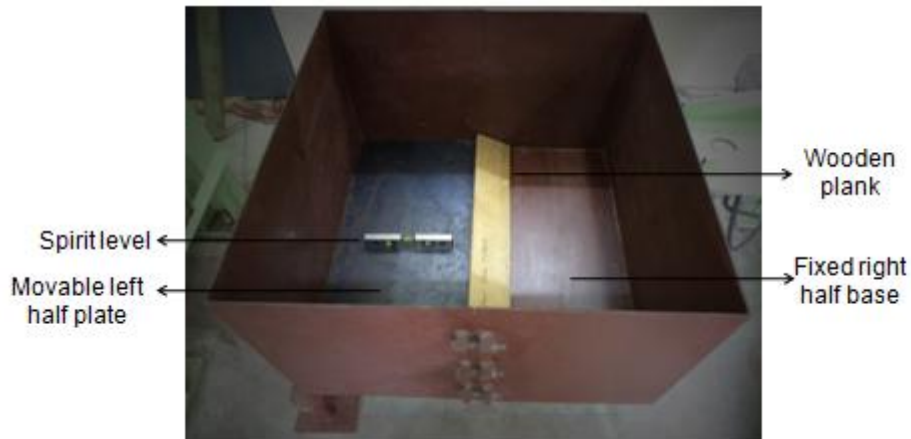
Figure 4.6: Base plates bridged with a wooden beam.
