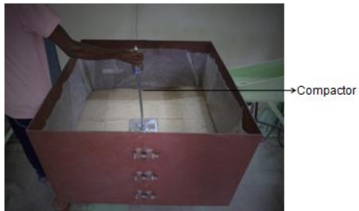
Figure 4.18: Compaction of sand layers.
