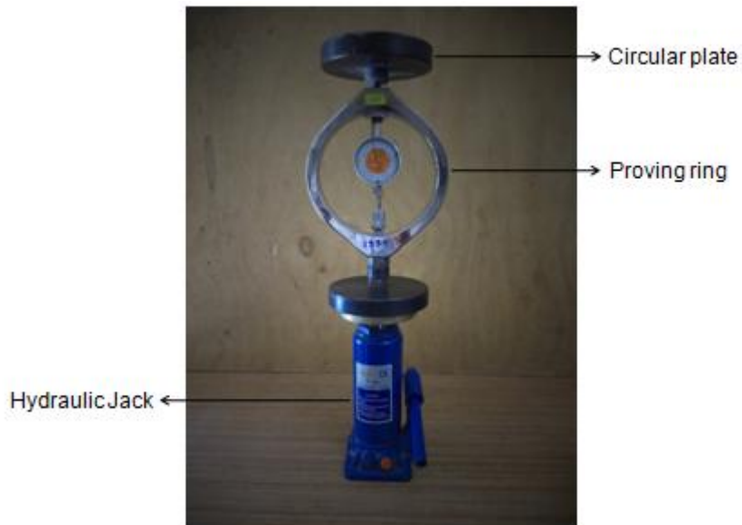
Figure 4.15: Hydraulic Jack with Proving ring
