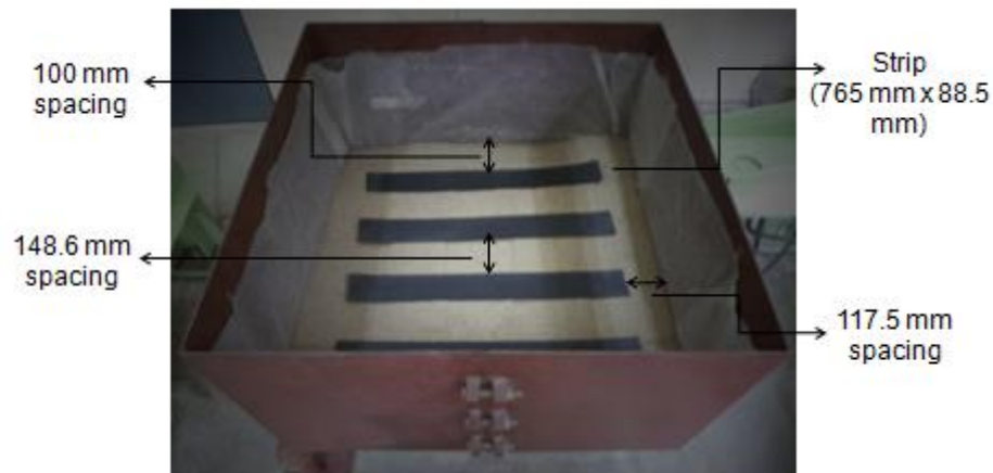
Figure 4.20: Placement of Paraweb Strips
