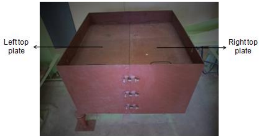
Figure 4.10: Placing of top plates
