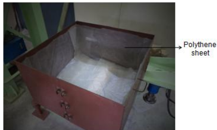
Figure 4.7: Inside of shear box covered with polythene sheet.
