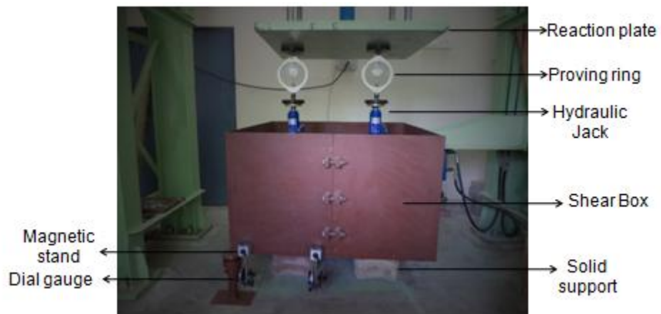
Figure 4.11: Front view of shear test apparatus
