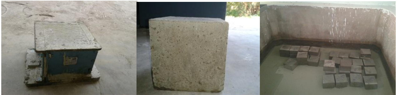
Figure 3.2 Preparation and curing of sample: (a) 150mm cube mould; (b) specimen after demolding; (c) Specimens being cured.
