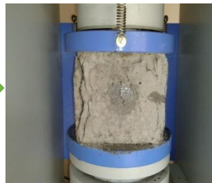
Figure 3.5(b) Failure pattern of the concrete cube
