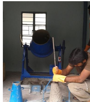
Figure 3.3 Slump measurement on fresh concrete
