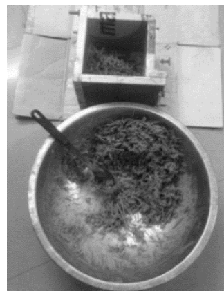
Figure 7. Chopped bagasse, lime, water and stone dust were mixed properly
