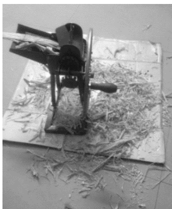
Figure 5. Dry sugarcane bagasse was chopped into fine pieces
