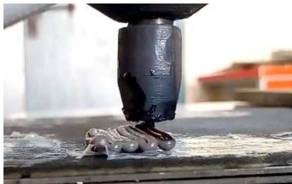
Figure 3-9 Sample being printed with a standoff distance of 3mm
