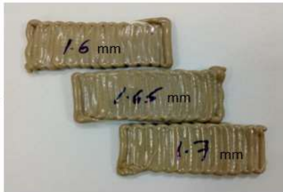
Figure 3-8 Specimens deposited with different road gap
