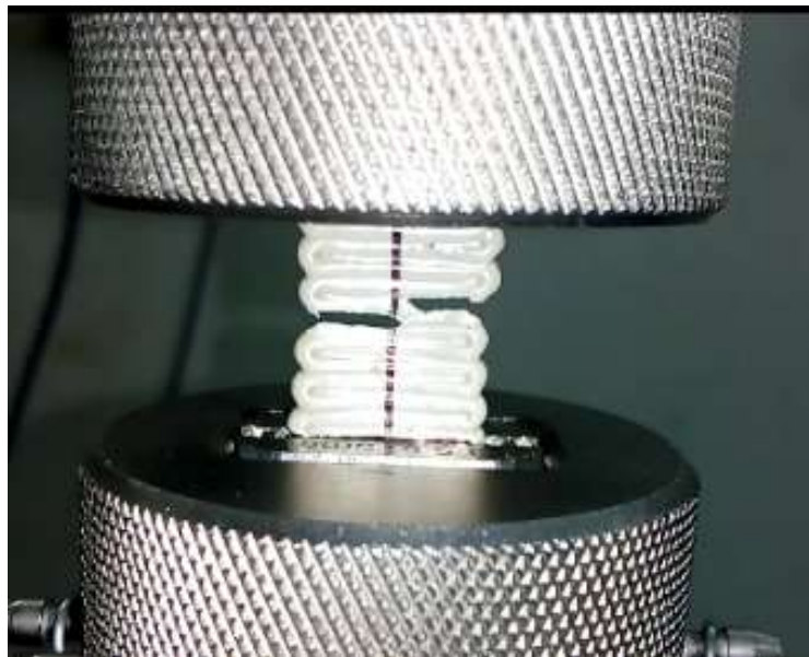
Figure 4-10 PEEK specimen testing with UTM
