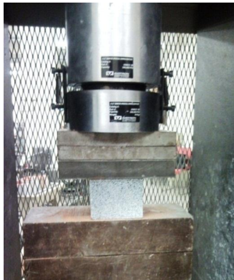
Fig 3.4: brick testing experimental setup
