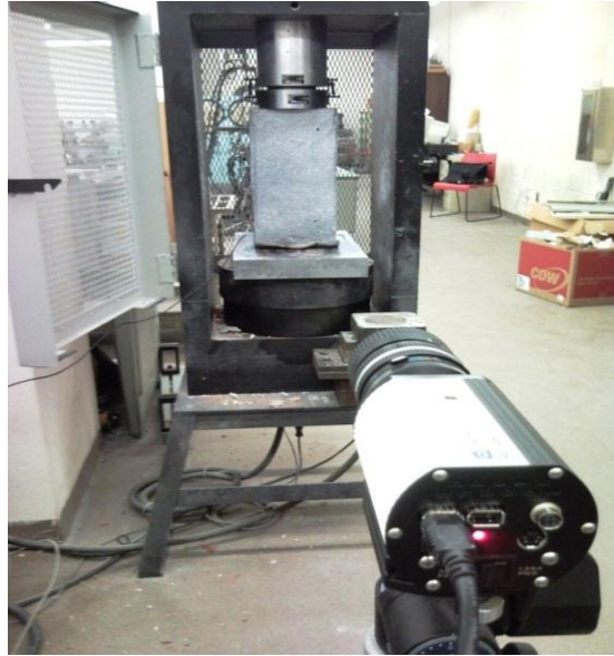
Fig 5.3: Experimental test setup for masonry testing
