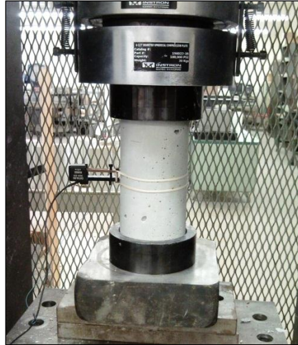
Fig 3.5: Photograph of mortar cylinder test setup
