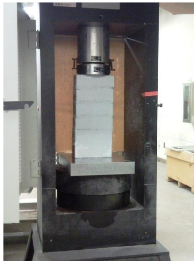
Fig 3.6: Photograph of the experimental setup for testing masonry
