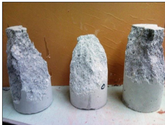
Fig 3.14: Photograph of the failed mortar specimens.
