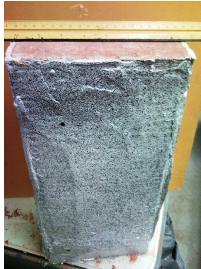
Fig 5.2 FRCM wrapped masonry specimen ready for testing
