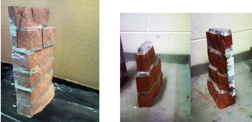
Fig 3.16: Photographs of the failed masonry specimens
