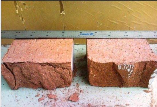
Fig 3.10: Failure of brick specimens
