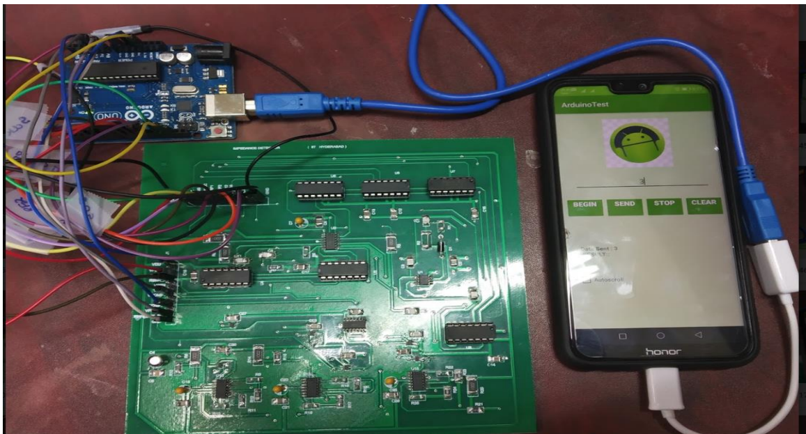
Figure 3-14 The board interfaced with cell phone and Arduino Uno
