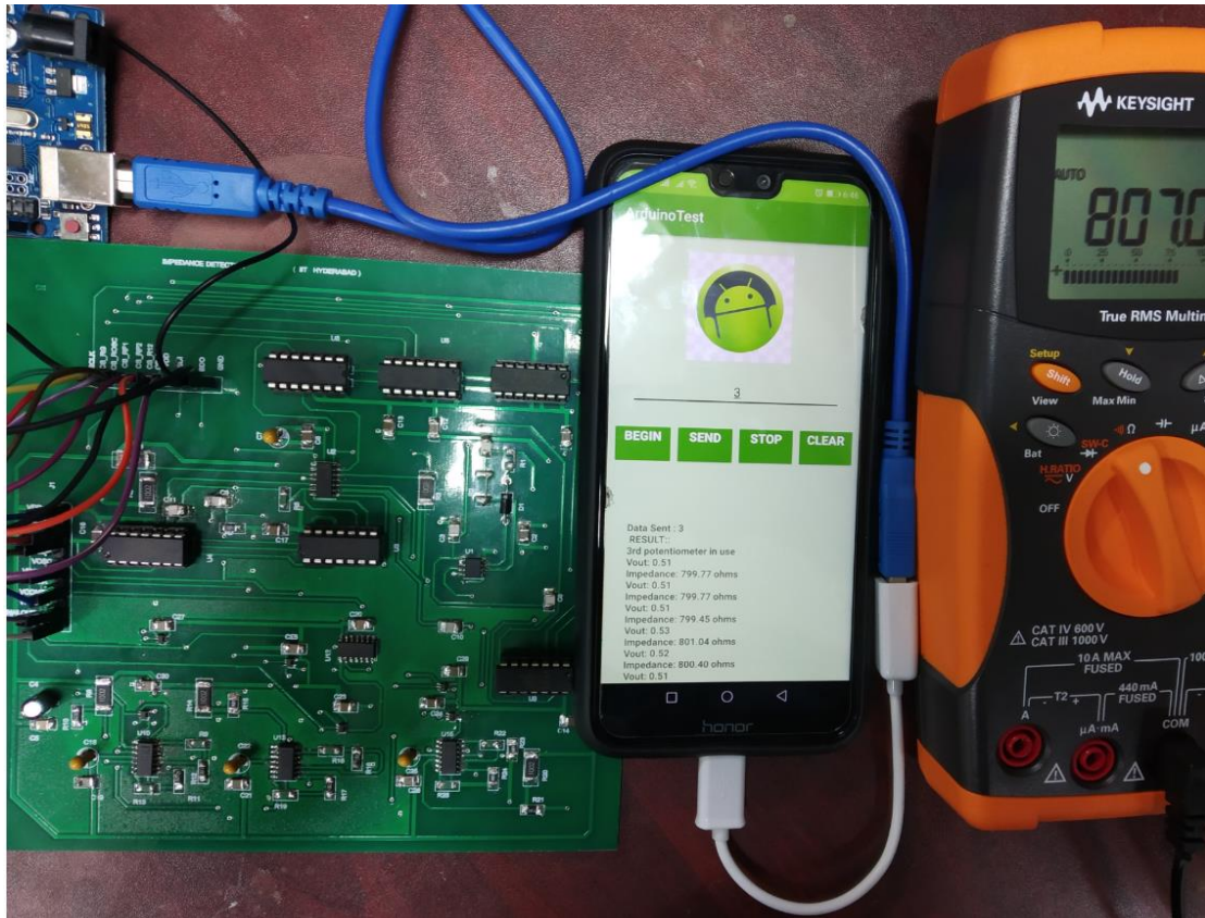
Figure 3-17 For a load of 807\Omega , 800\Omega displays on cell phone
