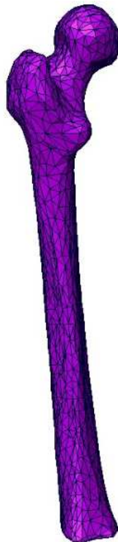
Fig 3.3. The 3D meshed model of Femur bone model with tetrahedral elements
