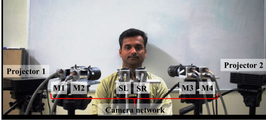
Figure 3.3: An instance of the oculofacial surface imaging platform used in this thesis. ‘SL’ and ‘SR’ cameras form a stereo pair. ‘Mi’ indicates i^{\text{th}} monocular camera.
