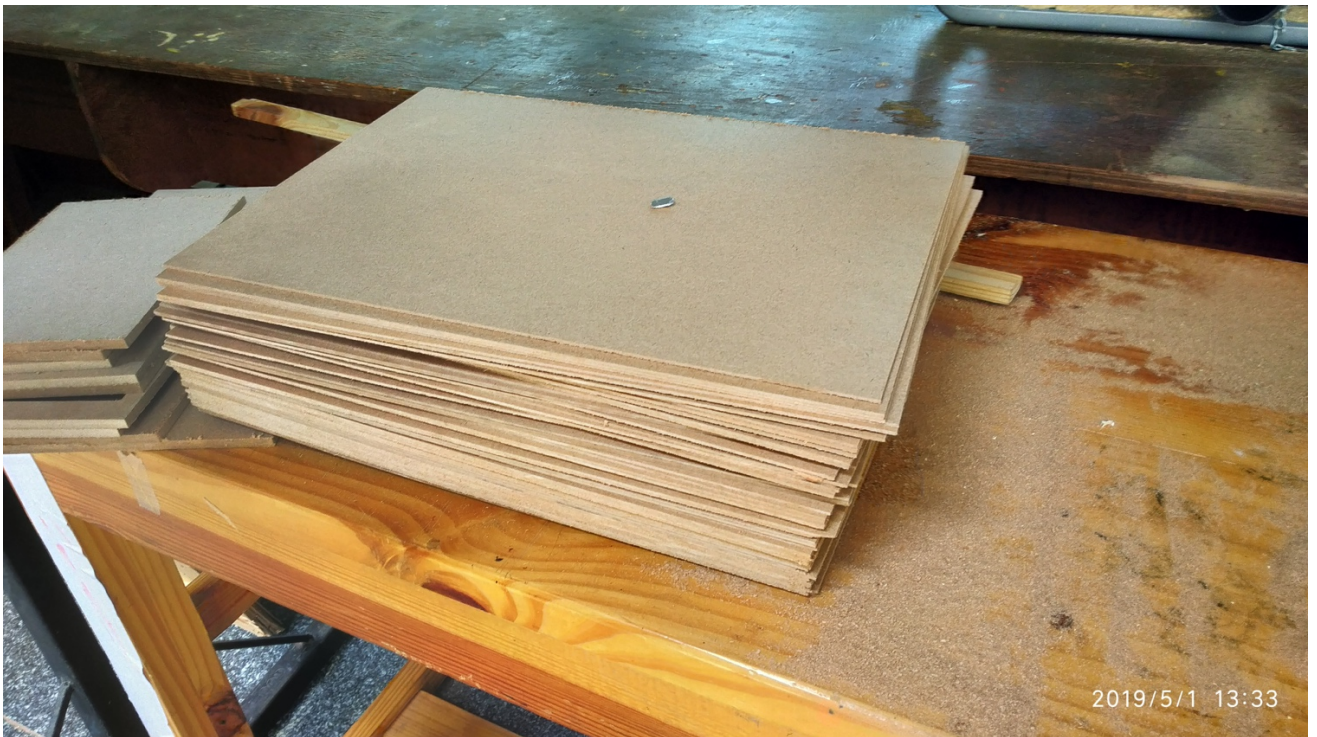
Fig1 61 6 mm mdf cut into A3 size with cutting machine
