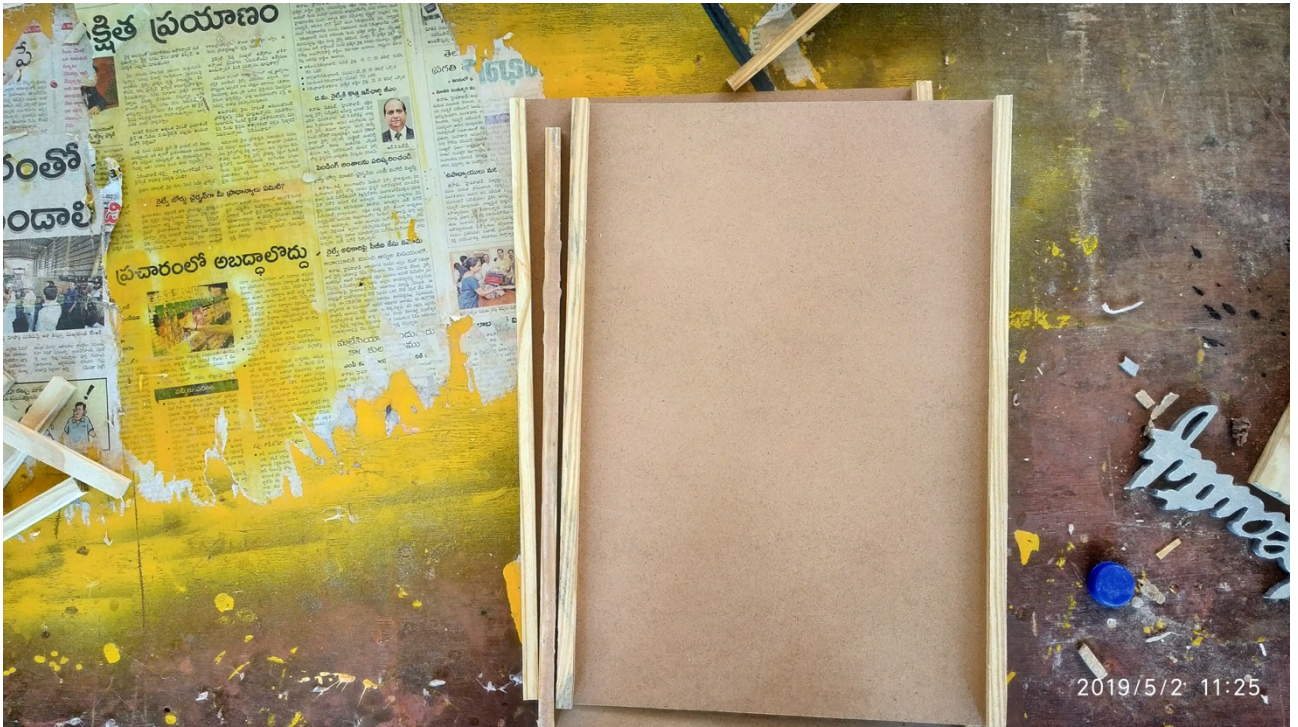
Fig1 64 sticking the wooden pieces with glue gun with MDF
