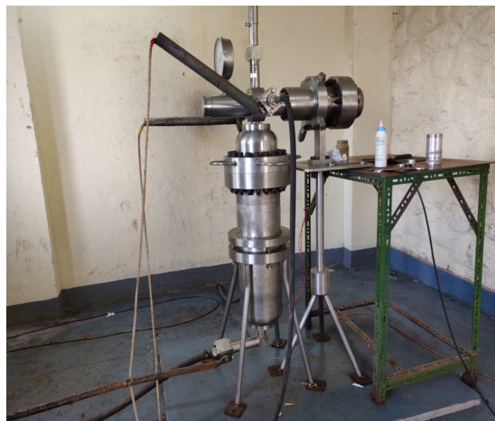
Figure 3.3: Ultrasonic burning rate test set up
