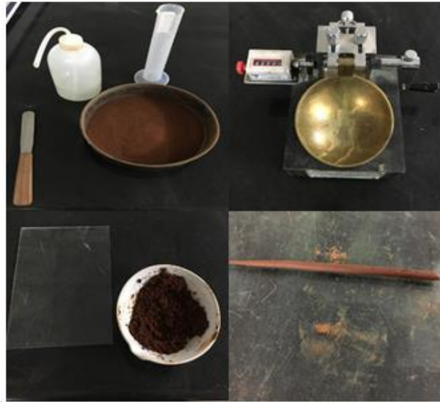
Figure 3.2a Images of the LL and PL test
