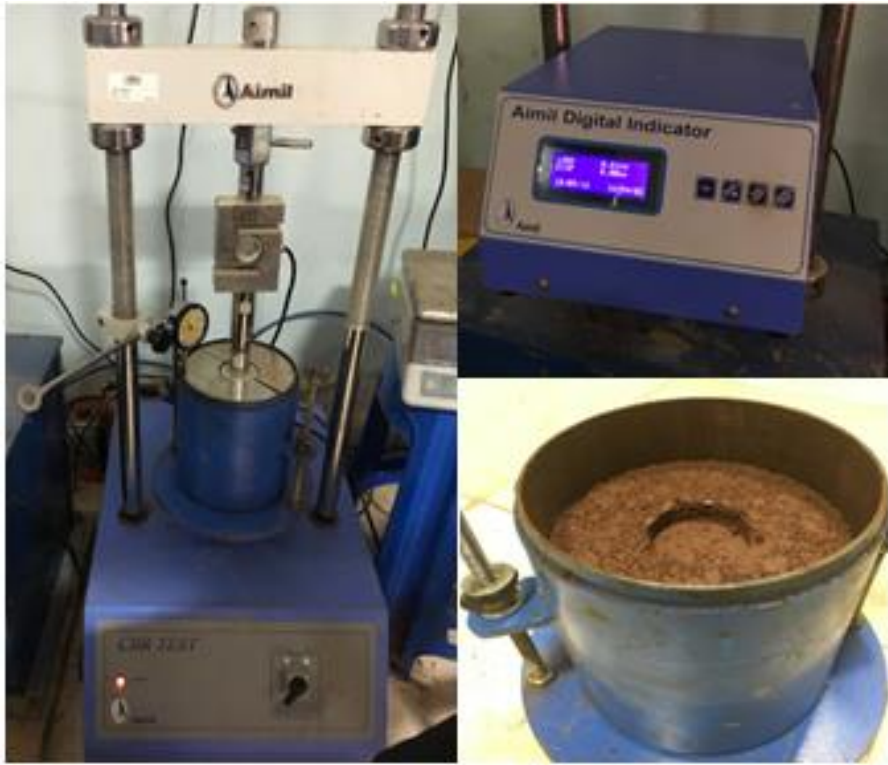
Figure 3.6a CBR setup and post test specimen
