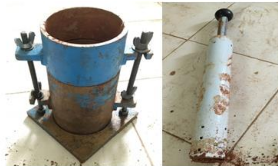
Figure 3.4 Mold and hammer used in standard proctor test
