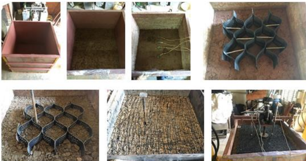
Figure 3.12 Various stages for the preparation of the test section
