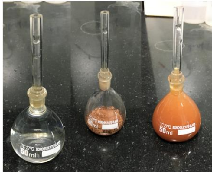
Figure 3.3 Specific gravity test by density bottle method
