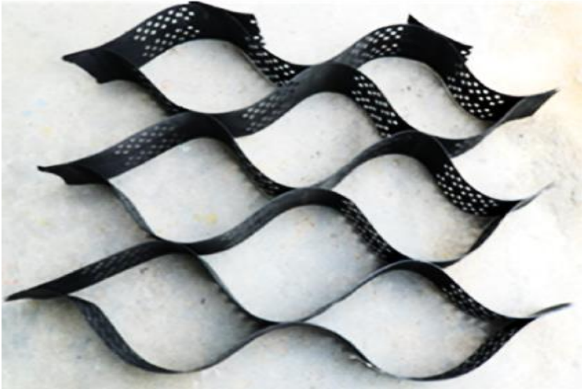
Figure 3.8 Typical geocell used in the study
