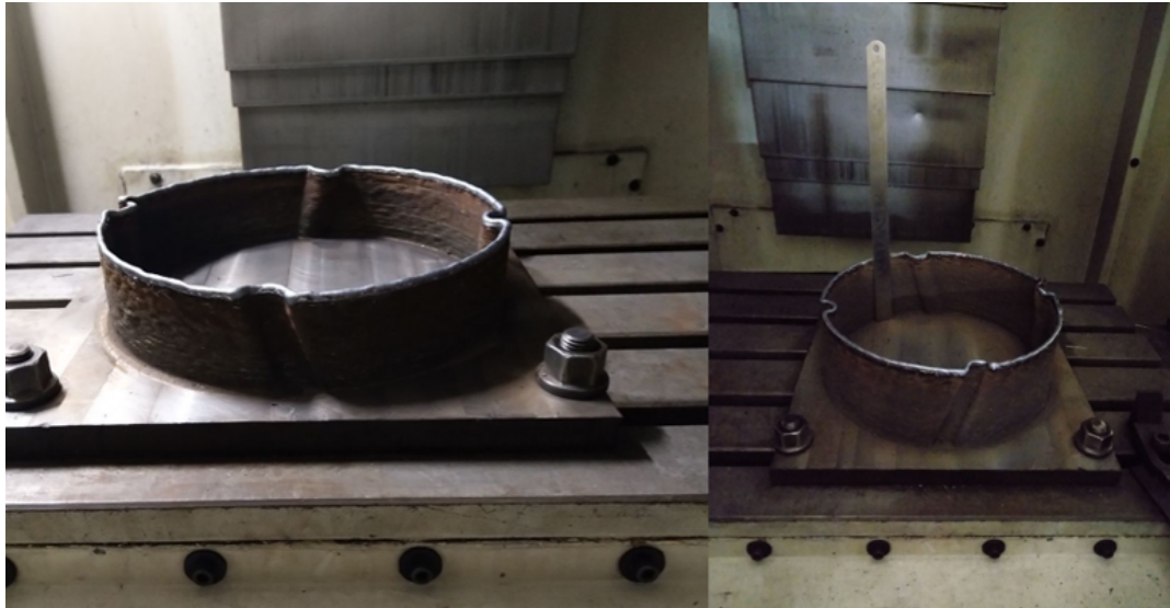
Figure 4.19: Deposition after layer 50 mm deposition and 100 mm deposition
