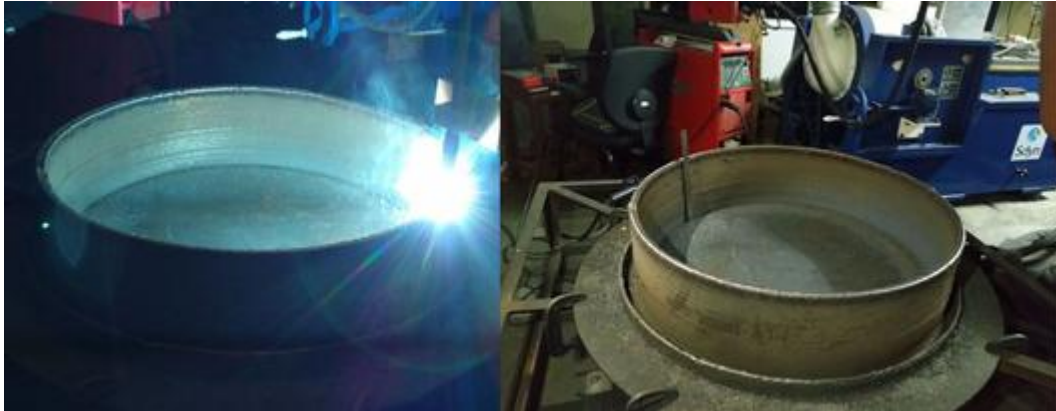
Figure 4.11: Last layer deposition on left and finally deposited layer with 900 mm diameter and 240 mm height with 20 mm wall thickness
