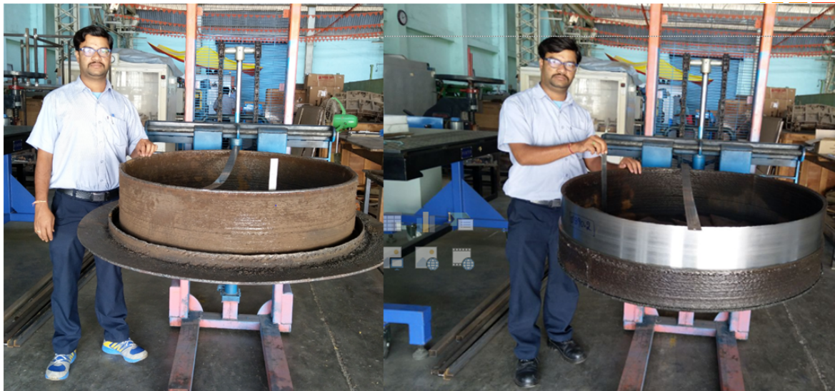
Figure 4.12: WAAM manufactured component before and after machining
