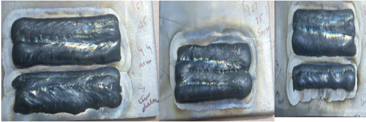
Figure 6.4: multi-pass IN625 deposition at low travel speed
