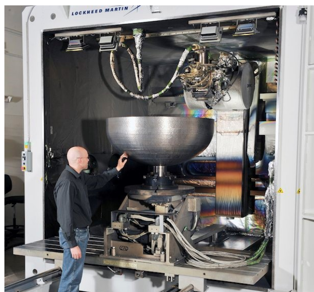
Figure 2.21: EBAM fabriacted component Ref- Lockheed Martin [13]
