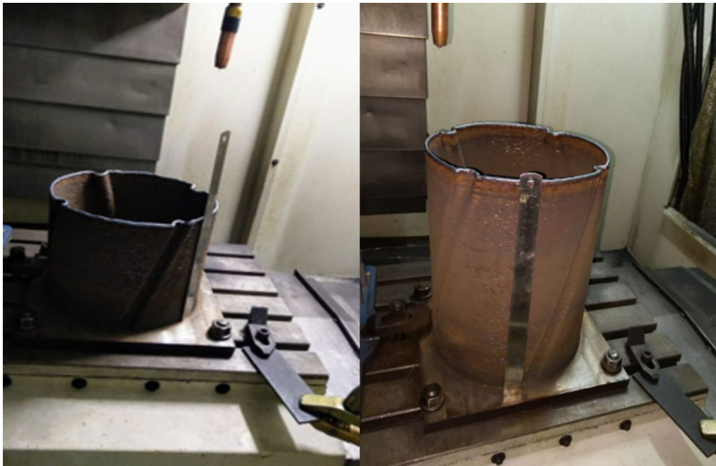
Figure 4.20: Deposition after layer 200 mm deposition and 300 mm deposition
