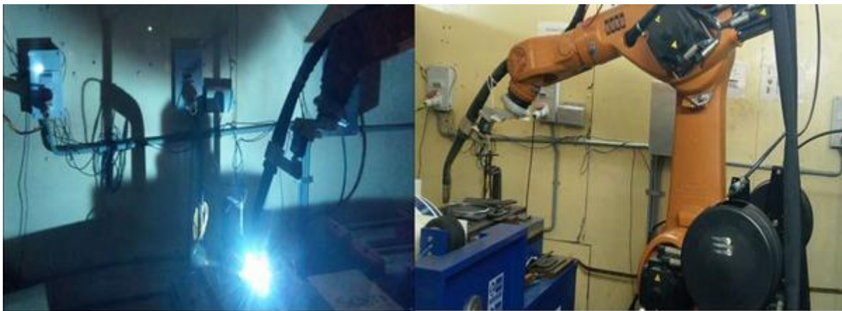
Figure 4.2: Fabrication process of medium scale components using Robotic WAAM
