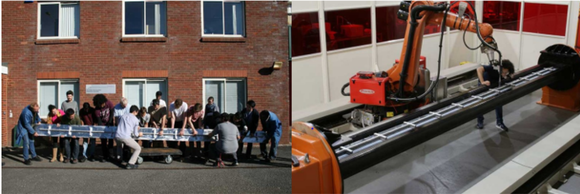
Figure 2.22: 6 m long Al alloy spar fabricated using Robotic WAAM [20]
