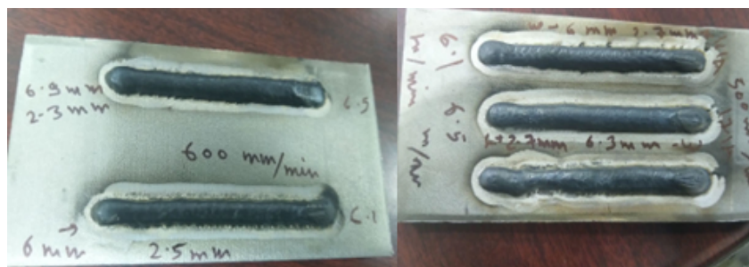
Figure 6.2: Single bead deposition of In625 on In600 plates
