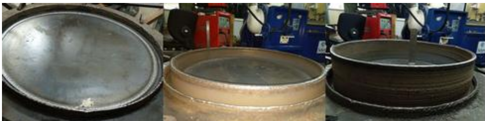
Figure 4.10: State of deposition after 1st layer,100 mm and 200 mm
