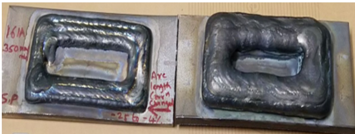
Figure 6.5: multi-pass IN625 deposition at low travel speed multi-pass(left) and multi-pass with multi-layer(3*3)
