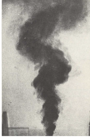
Figure 2.3: Plane turbulent plume showing large scale motions [1]
