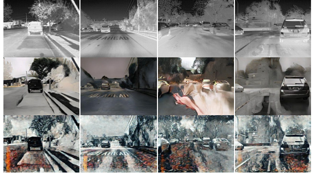
Figure 6. Row 1: Thermal images from FLIR ADAS[13] dataset; Row 2: Translations generated using UNIT[25]; Row 3: Translations generated using CycleGAN[40].
