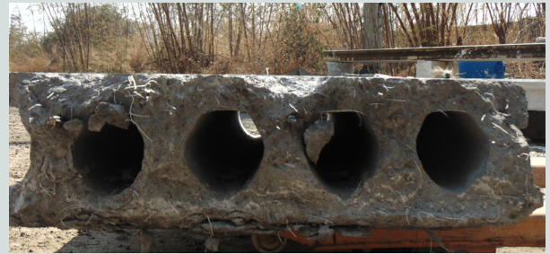
Figure 8. Cross section of hollow-core slab showing even macrosynthetic fiber distribution.
