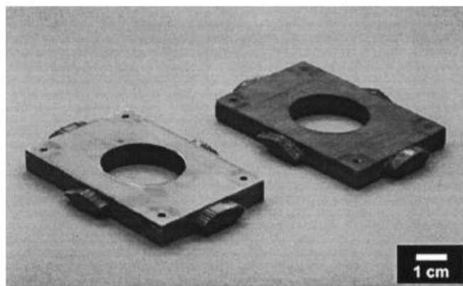
Figure 2.27. Examples of unidirectional glass fiber /epoxy composite parts built with LOM. The part on the right has been post-cured (Klosterman et al. 1998).
