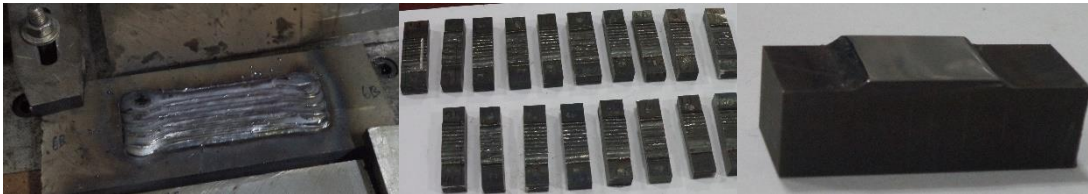
Figure 6.1. Specimen preparation (a) weld-deposition (b) cross-sectional cut weld specimen (c) a cut-specimen with polished top surface for hardness measurement.
