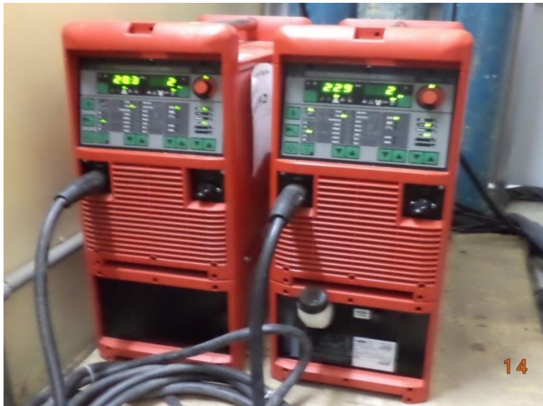
Figure 3.5. Complete welding system based on the power source Time Twin Digital 5000.
