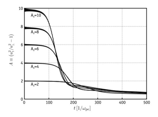
Observe that irrespective of the initial degree of anisotropy, the system saturates to a non zero threshold value. Our original problem described with appropriate boundary conditions mandates that waves longer than the linear size of the domain cannot exist, which explains the residual anisotropy.
