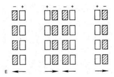
The open rectangles correspond to the ion fluid elements, while the darkened ones represent the electron fluid elements. The resulting grouping of charges causes the development of a periodic **E** field in space, which tries to restore the electrons to their original positions.
