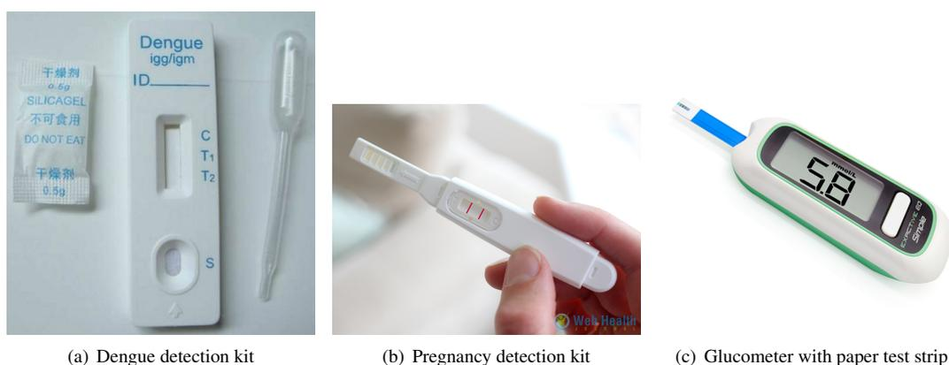
Figure 1.4: Paper based diagnostic devices.
