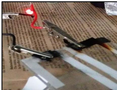
Figure 5.15: Paper cell illuminating LED
