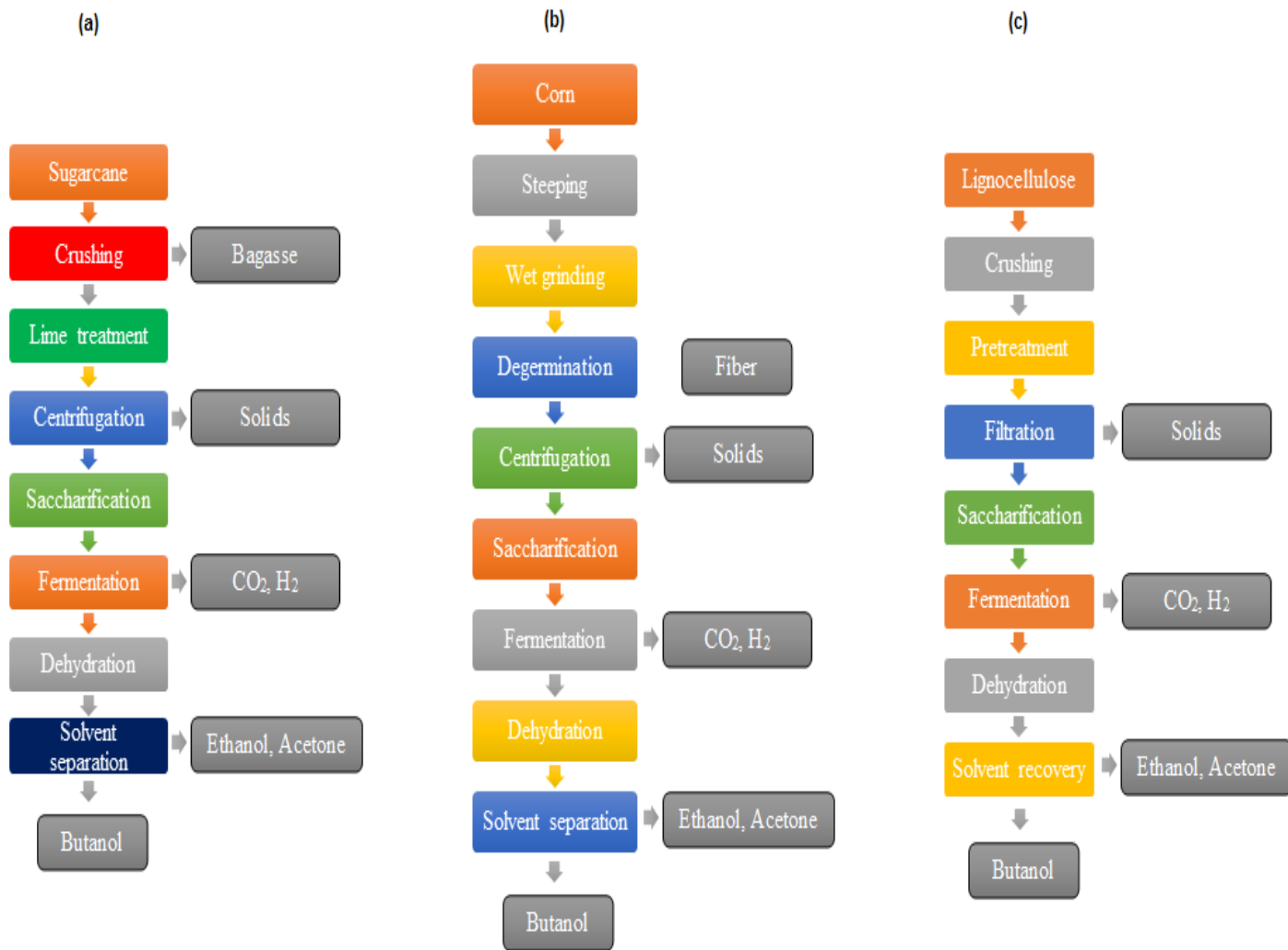
Figure 3.1. Schematic process flow diagram for production of butanol [Manish Kumar et al., 2012].
