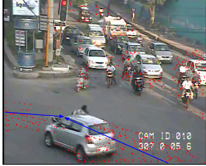
Figure 8.13: The intersection of two trajectories during an accident. The trajectories of the motorcycle and car intersect each other also there is no further progress in the trajectories of the motorcycle and car, thus considered as a collision.
