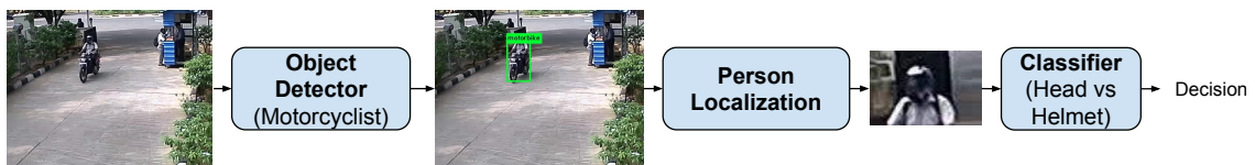
Figure 8.2: Block diagram of proposed framework for the detection of motorcyclists without helmet.
