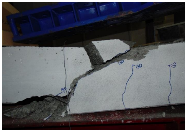
c) The failure mode of the SF00-1 specimen
