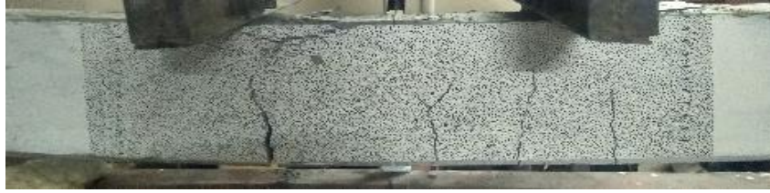
Figure 5.24: Flexure behavior of HB100 specimen
