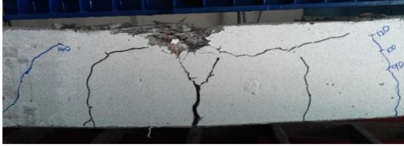
Figure 5.5: Flexure failure of SF35 specimen
