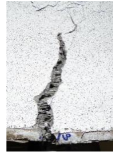
b) crack bridging action of PO fibers
