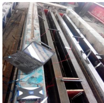
b) Strand strain measurement during pretensioning
