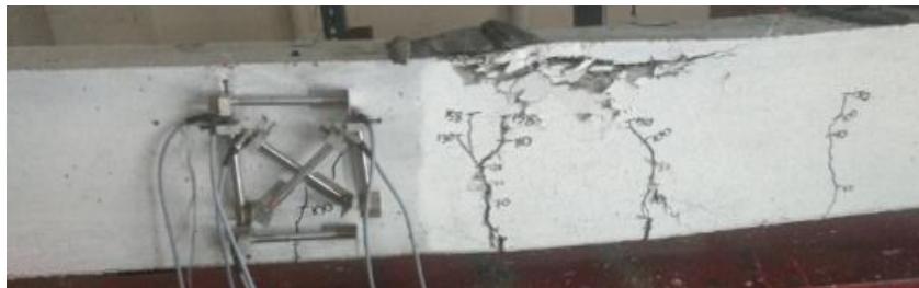
Figure 5.9: Flexure failure of SF100 specimen
