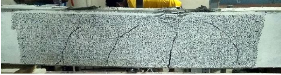
Figure 5.20: Flexure behavior of HB35 specimen
