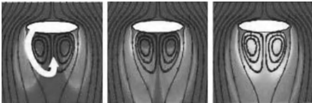
Figure 8.10 Snapshots of the computed developing concentration of the product in the wake of a bubble in a gas–liquid–solid reaction. Reproduced from Raffensberger et al. [122]
