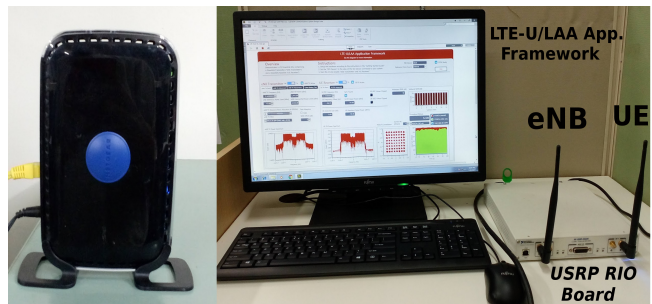
Fig. 3. Equipment used in the testbed: (i) Netgear N600 wireless dual band router WNDR3400v3 used as Wi-Fi AP. (ii) USRP RIO board with LTE-U eNB and LTE-U user operated using LTE-U/LAA Application framework.
