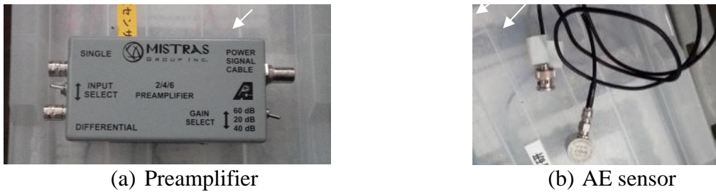
281 Figure 2: Flexural Test Setup with Acoustic Emission Sensors 282
